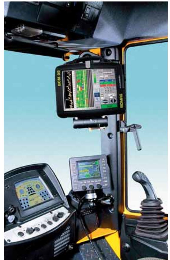
The cab of this Bomag BW213-4 BVC roller, which is fitted with the company's VarioControl system — an IC system for soil machines, incorporates the machine's basic control panel (center), the VarioControl operating panel (lower right) and the Bomag documentation system (upper right).
