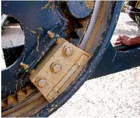
Indicative of today's easier-to-service machines, this Deere grader features circle wear inserts (alloy or nylon) that are designed for replacement in about two hours using only a 9/16-inch wrench.
