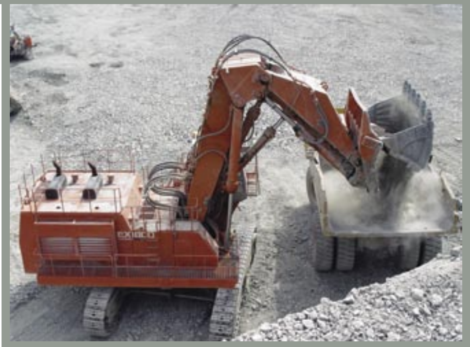
Right: A Hitachi EX1800 shovel loads shot rock into a Caterpillar 777C haul truck at the base of the cliff.
